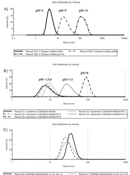
Figure 2. Self aggregation behavior of selected poly(DEAEM-b-MAOB) blockcopolymers: A.-1 mg/mL solution of poly(DEAEM-b-MAOB)  $M_w = 33,080$  g/mol, 67%DEAEM at different pH-values. B.-1 mg/mL solution of poly(DEAEM-b-MAOB)  $M_w = 64,000$  g/mol, 81%DEAEM at different pH-values. C.-1 mg/mL solution in Buffer (pH 7.4) of poly(DEAEM-b-MAOB)  $M_w = 64,000$  g/mol, 81%DEAEM at different salt concentration.
