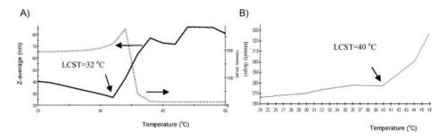
**Figure 4.**Determination of the lower critical solution temperature (LCST) of NIPAAm copolymers by DLS: A.- Poly(NIPAAm-b-HA) of 26 Kg/mol in water. B.- Poly(NIPAAm-co-MD4) of 31.8 Kg/mol in buffer of pH 7.4
