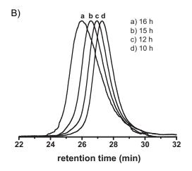
Figure 3. Kinetics of RAFT polymerization of NIPAAm using 4-cyanopentanoic acid dithiobenzoate as CTA in p-Dioxane at 70 °C: A.- Evolution of molecular weight ( $M_n$ ) and polydispersity (PDI) with conversion. B.-GPC traces from refractive index detector at different polymerization times.
